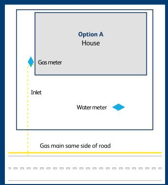
as a straight line between the tapping point and the meter.
